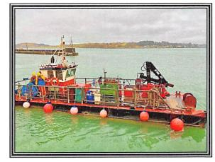
The Commissioners own and operate the grab hopper dredger MV Mannin. The vessel operates mainly at Padstow on maintenance dredging but she has proved to be very versatile and is available for hire for work at other ports. During 2021 the Mannin undertook a complete overhaul to pass her MCA load line inspection with the Commissioners investing in a new grab to complement the works.
